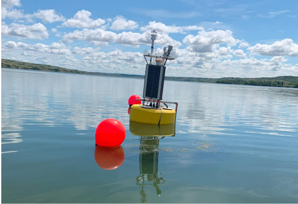
Newly deployed SuperBuoy for water quality monitoring at Buffalo Pound Lake, SK; Saskatchewan Water Chemistry and Ecology Laboratory
