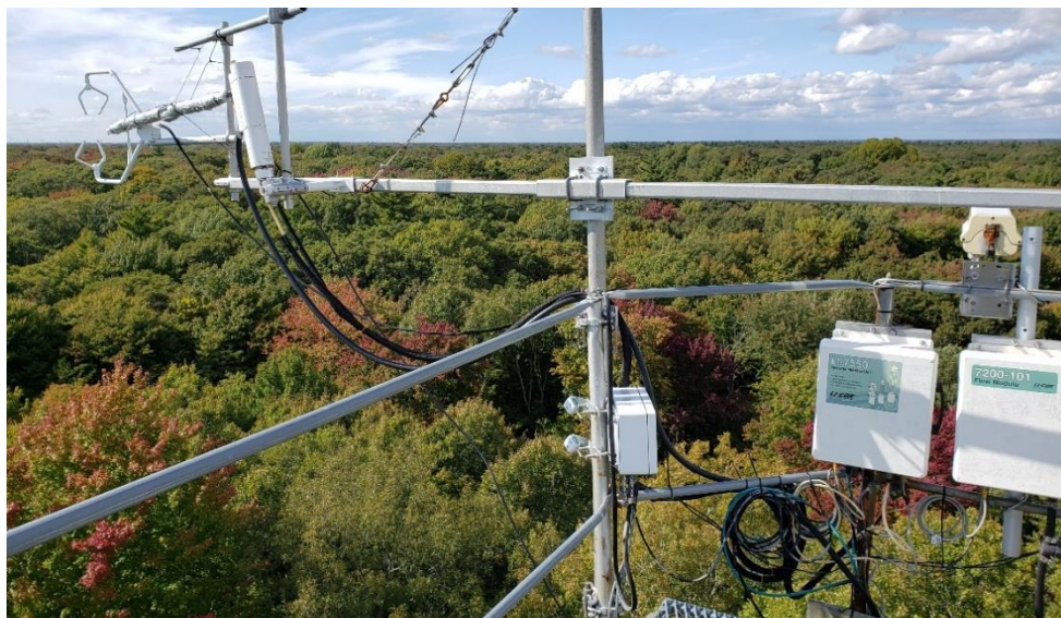
Eddy covariance instrumentation on top of flux tower at the Turkey Point Environmental Observatory, ON, operated by McMaster University
