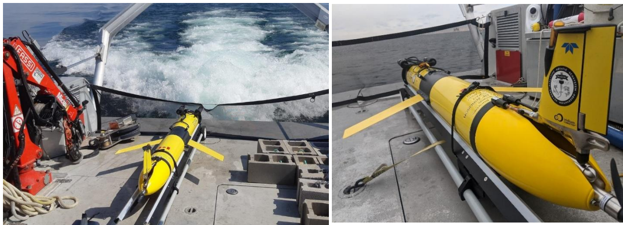
Above: Slocum autonomous glider for deployment in Lake Ontario to measure water quality parameters; part of the Real-Time Aquatic Ecosystem Observation Network (RAEON), led by the University of Windsor
